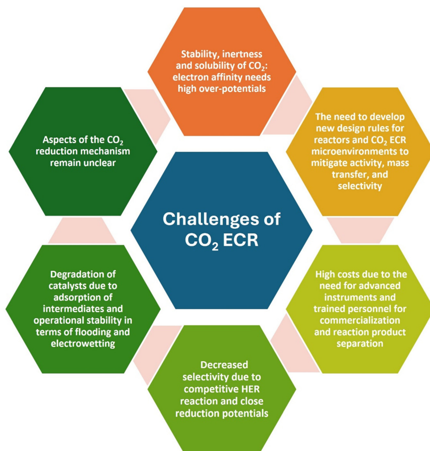
Scheme 1 Challenges during the ECR of \text{CO}_2 .
