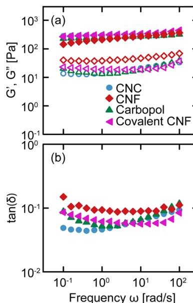
Fig. 2 (a) Storage (closed symbols)  $G'$  and loss (open symbols)  $G''$  moduli and (b)  $\tan(\delta) = G''/G'$  as a function of frequency  $\omega$  for the four classes of gels: CNC, entangled CNF, Carbopol, and covalent CNF.
