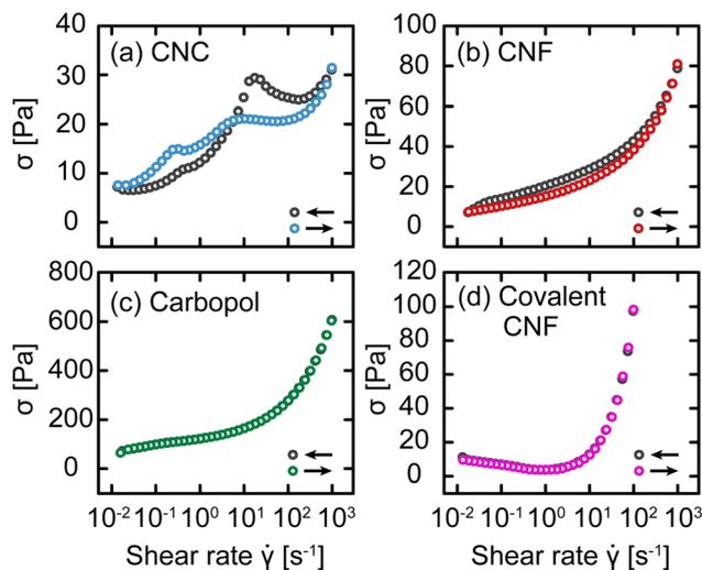
Fig. 8 Stress  $\sigma$  as a function of shear rate  $\dot{\gamma}$  for (a) CNC, (b) entangled CNF, (c) Carbopol, and (d) covalent CNF gels with decreasing  $\dot{\gamma}$  (gray) and increasing  $\dot{\gamma}$  (color) with  $\delta t = 10$  s.
