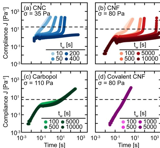
Fig. 5 Compliance  $J = \gamma/\sigma$  as a function of time at constant stress  $\sigma$  for various waiting times  $t_w$  after yielding for (a) CNC, (b) entangled CNF, (c) Carbopol, and (d) covalent CNF gels. Dashed lines indicate the creep threshold  $J^*$  used to identify the yield time  $\Delta t_y$ .
