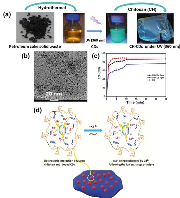
Fig. 6 (a) Synthesis process of CQDs and CQDs-CH from petroleum coke residues, (b) TEM image of CQDs, (c) extraction efficiency at different times for  $\text{Cd}^{2+}$  using CH and CH-CQDs in the dark and under UV light (360 nm) at pH = 8, and (d) mechanism of cation exchange in the presence of  $\text{Cd}^{2+}$  of the CH-CQDs membrane. Reproduced (adapted) with permission from ref. 97. Copyright© 2020, Environmental Sciences Europe.
