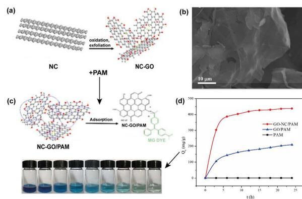
**Fig. 8** (a) Synthesis process of GO derived from petroleum coke (GO-NC), (b) SEM image of GO-NC, (c) process of obtaining the PAM/GO-NC hydrogel and adsorption of the MG dye, and (d) adsorption capacity of GO-NC/PAM, GO/PAM and PAM. Reproduced (adapted) with permission from ref. 152. Copyright© 2018, Taylor & Francis.
