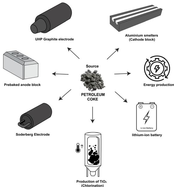
Fig. 2 Different applications of petroleum coke as a carbon source.
