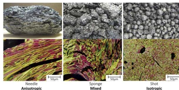
Fig. 3 Petroleum coke types and optical textures. Reproduced (adapted) with permission from ref. 24. Copyright© 2015, The Minerals, Metals & Materials Society.
