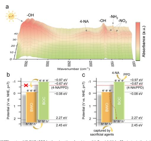
Fig. 8 (a) In situ DRIFTS spectra of 10-BWO@BOC for the adsorption of a mixture of H<sub>2</sub>O and 4-NA for 20 minutes in the dark and under UV-vis light irradiation for another 20 minutes. The proposed charge transfer mechanism of (b) type-II and (c) Z-scheme heterostructures over the 10-BWO@BOC heterostructure for the photocatalytic hydrogenation reaction of 4-NA under UV-vis light irradiation.
