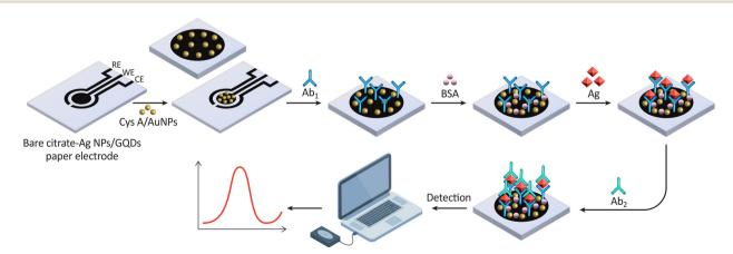
Fig. 17 This illustration shows the steps for fabricating a paper-based electrochemical biosensor. It begins with a bare electrode modified with AgNPs and GQDs, followed by Ab immobilization, blocking with BSA to prevent non-specific binding, Ag capture, and finally, detection with a secondary antibody (Ab2), leading to signal generation for analysis. Reproduced from ref. 222. with permission from [Elsevier], copyright [2020].
