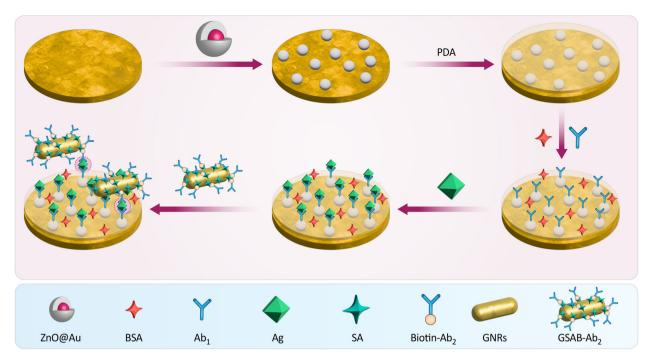
Fig. 13 The scheme illustrates the assembly of a SPR biosensor, starting with a ZnO@Au nanocomposite base layer. Bovine serum albumin (BSA) and primary antibodies (Ab1) are applied to capture Aq, followed by SA and biotin-Ab2 to enhance the signal. GNRs and GSAB-Ab2 are then introduced for signal amplification, creating a sensitive, sandwich-type biosensor for detecting hlgG. Reproduced from ref. 199 with permission from [Elsevier], copyright [2022].
