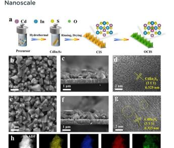
Fig. 1 (a) The synthetic schematic for the OCIS photoanode. The topview SEM images of (b) CIS, and (e) OCIS. The cross-sectional SEM images of (c) CIS and (f) OCIS. HRTEM images of (d) CIS and (g) OCIS. (h) EDS mapping of OCIS.
