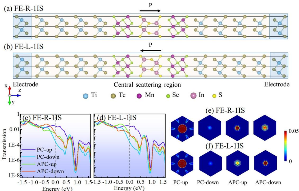
**Fig. 2** The structure schematic diagrams of the MFTJ with (a) FE-R-1IS and (b) FE-L-1IS states. The spin-dependent zero-bias transmission coefficient curves of the MFTJ with (c) FE-R-1IS and (d) FE-L-1IS states. The spin-dependent  $k_{||}$ -resolved transmission spectra of the MFTJ with (e) FE-R-1IS and (f) FE-L-1IS states.
