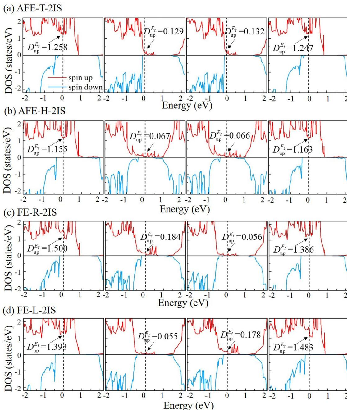
Fig. 5 The spin-dependent DOS of the  $\text{Mn}_2\text{Se}_3/\text{bilayer-In}_2\text{S}_3/\text{Mn}_2\text{Se}_3$  part in the MFTJ with (a) AFE-T-2IS, (b) AFE-H-2IS, (c) FE-R-2IS and (d) FE-L-2IS states.  $D_{\text{up}}^{E_f}$  represents the spin-up DOS value at the Fermi level.
