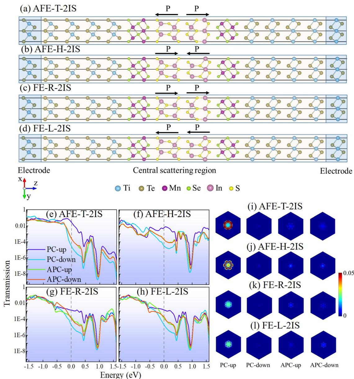
**Fig. 3** The structure schematic diagrams of the MFTJ with (a) AFE-T-2IS, (b) AFE-H-2IS, (c) FE-R-2IS, and (d) FE-L-2IS states. The spin-dependent zero-bias transmission coefficient curves of the MFTJ with (e) AFE-T-2IS, (f) AFE-H-2IS, (g) FE-R-2IS, and (h) FE-L-2IS states. The spin-dependent  $k_{||}$ -resolved transmission spectra of the MFTJ with (i) AFE-T-2IS, (j) AFE-H-2IS, (k) FE-R-2IS, and (l) FE-L-2IS states.
