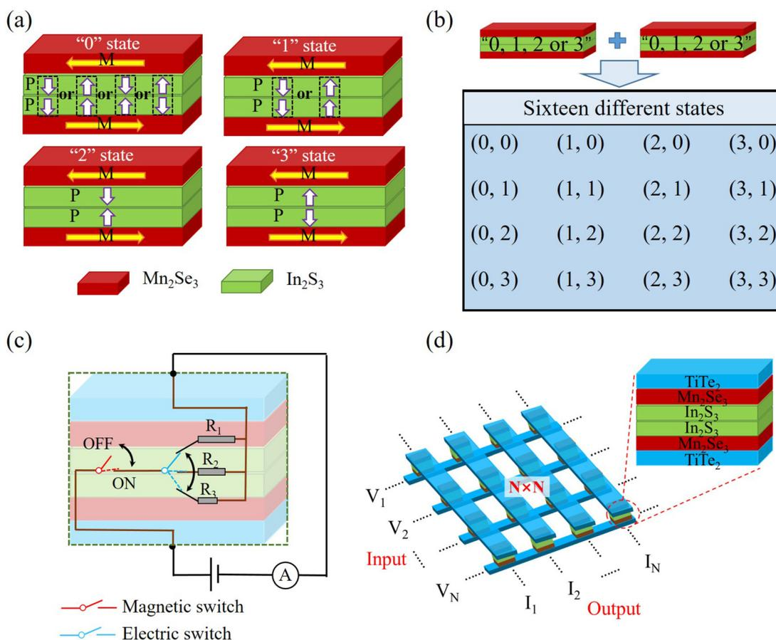
**Fig. 6** The multilevel storage mechanism of (a) four distinguishable conductance states in a MFTJ unit, and (b) sixteen different states achieved by two series MFTJ units. The in-memory computing application mechanism of (c) the equivalent circuit diagram for magnetic and electric switch, (d) the  $N \times N$  MFTJ array units.
