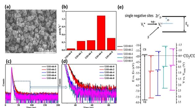
Fig. 6 (a) SEM images of UiO-66-6 and UiO-66-0 (inset). (b) Results of CO production from photocatalytic CO<sub>2</sub> production under visible light illumination over various UiO-66-*X*. (c and d) Time-resolved PL spectra of various UiO-66-*X*. (e) Proposed mechanism of the energetic state of missing ligands and derived band structure for various UiO-66-*X* (*X* = 0, 2, 4, 6, 8). Reproduced with permission from ref. 43. Copyright 2022, American Chemical Society.
