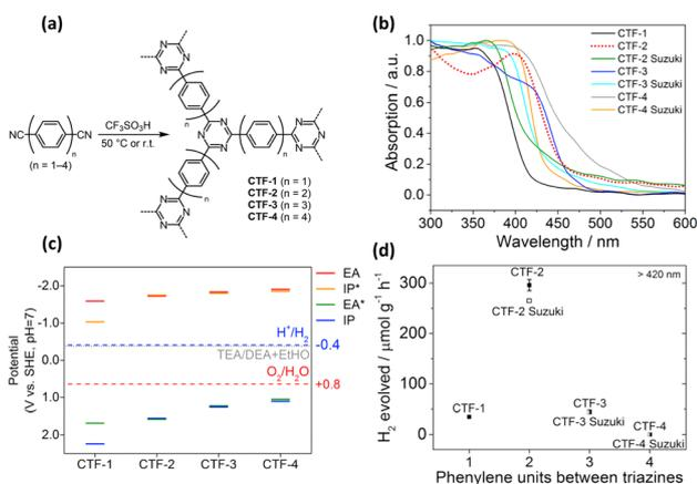
**Fig. 14** (a) Synthesis of CTF-*n* *via* acid-catalyzed cyclotrimerization. (b) Corresponding absorption spectra. (c) Calculated reducing (EA, IP\*) and oxidizing potentials (IP, EA\*) for CTF-3. (d) Relationship between H<sub>2</sub> yield and number of repeating phenylene units for CTF-*n*. Reproduced with permission from ref. 115. Copyright 2017, Elsevier.
