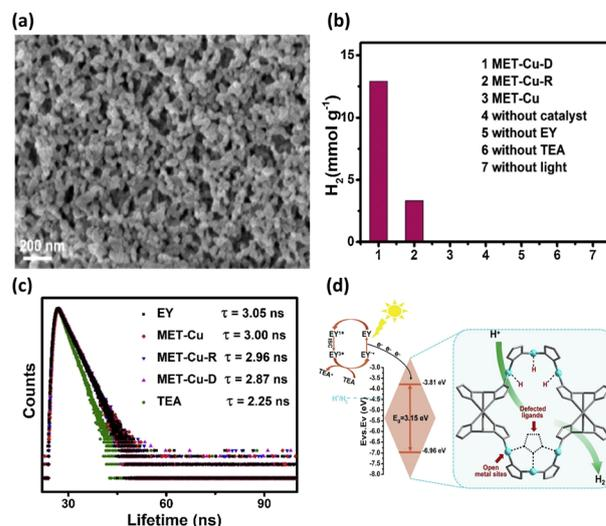
Fig. 5 (a) SEM images of MET-Cu-D and MET-Cu (inset). (b) Results of photocatalytic H<sub>2</sub> production under visible light illumination over the three samples under different conditions. (c) Time-resolved PL spectra of EY in the presence of the three samples. (d) Proposed mechanism of interfacial charge transfer for MET-Cu-D. Reproduced with permission from ref. 42. Copyright 2021, Elsevier.
