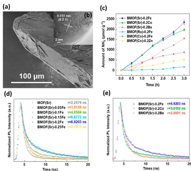
Fig. 1 (a) SEM and (b) HRTEM images for BMOF(Sr)-0.2Fe. (c) Results of photocatalytic  $\text{NH}_3$  synthesis under white light illumination on various BMOFs samples. (d) Time-resolved PL data of MOF(Sr) and various BMOF(Sr) samples. (e) Time-resolved PL data of BMOF(Sr)-0.2Fe, BMOF(Sr)-0.2Co and BMOF(Sr)-0.2Ba. Reproduced with permission from ref. 37. Copyright 2021, American Chemical Society.
