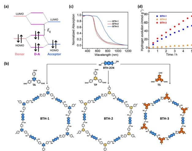
**Fig. 15** (a) Diagram of molecular orbital interaction between donor and acceptor moieties and the formation of a new bandgap in D–A components. (b) Synthetic procedures of BTH-1, BTH-2, BTH-3. (c) Corresponding absorption spectra. (d) Results of photocatalytic H<sub>2</sub> production under visible light illumination over the three samples. Reproduced with permission from ref. 116. Copyright 2022, Springer Nature.
