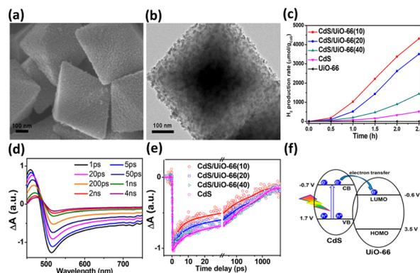
Fig. 7 (a) SEM and (b) TEM images of CdS/UiO-66(10). (c) Results of photocatalytic  $H_2$  production under visible light illumination over five relevant samples. TA spectra of (d) pure CdS. (e) Comparison of kinetics profiles probed at 650 nm among pure CdS and the three CdS/UiO-66. (f) Proposed mechanism of interfacial charge transfer for CdS/UiO-66. Reproduced with permission from ref. 92. Copyright 2019, American Chemical Society.
