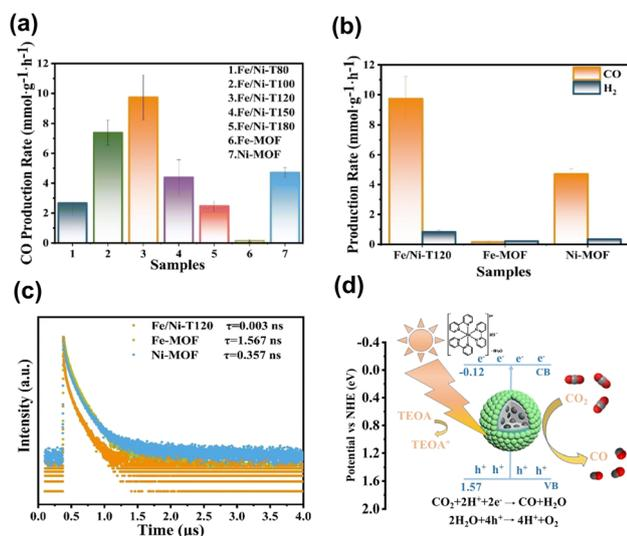
Fig. 13 (a and b) Results of CO and H<sub>2</sub> production from photocatalytic CO<sub>2</sub> production under visible light illumination over relevant samples. (c) Time-resolved PL spectra of relevant samples. (d) Proposed mechanism of photocatalytic CO<sub>2</sub> reduction on Fe/Ni-T120. Reproduced with permission from ref. 100. Copyright 2012, American Chemical Society.
