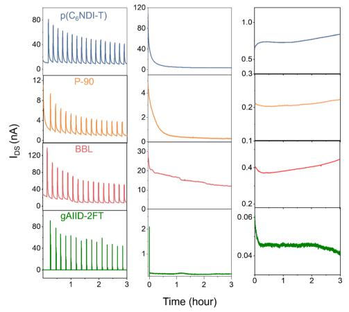
Fig. 5 The stability of OPECTs. Left: The channel current of the OPECT monitored over three hours ( $V_{DS} = V_{GS} = 0.4 \text{ V}$ ) under light pulses (ON for 1 min, OFF for 10 min) middle: in the dark. The polymer gates were used. Right: The channel current of the OPECT monitored over three hours in the dark ( $V_{DS} = V_{GS} = 0.4 \text{ V}$ ), where Ag/AgCl was used as a gate and p(C<sub>6</sub>NDI-T), P-90, BBL and gAIID-2FT used as a channel of OECTs.
