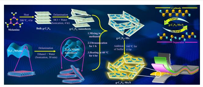
Scheme 1 Schematic illustration for the synthesis of g-C<sub>3</sub>N<sub>4</sub>-Mx/S nanocomposites and the structure of pouch cell demonstrating arrangements of electrodes and a separator.
