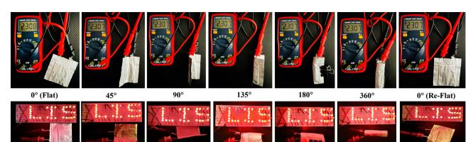
Fig. 6 Upper row: digital pictures of the OCV for the pouch cell consisting of the  $g-C_3N_4-Mx/S$  cathode at different folding angles. Bottom row: pictures of LEDs lighten up by a pouch cell at different folding angles demonstrating the excellent flexible feature of the developed pouch cell.
