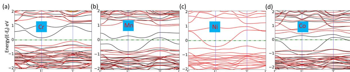
**Fig. 5** (a)–(d) Band structure of Cr, Mn, Ni, and Co-doped SiP<sub>2</sub> monolayers, respectively.
