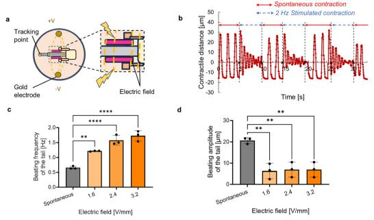
Fig. 5 Evaluation of the controllability of the biohybrid self-beating actuator. (a) Schematic diagram of the electric field application to the biohybrid self-beating actuator. (b) Temporal beating displacement of the tail when the electric field is intermittently applied. (c) Beating frequency and (d) beating amplitude of the tail when the electric field is applied. Bars represent the mean  $\pm$  SEM. \*\*p < 0.005, \*\*\*\*p < 0.0001, Tukey-Kramer
