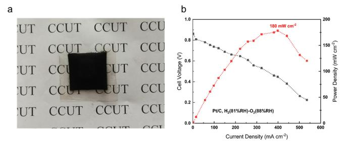
Fig. 9 (a) PTI-N-100 membrane electrode physical photo; (b) single-cell performance of AEMFCs with PTI-N-100 membranes at a cell temperature of 80 °C.
