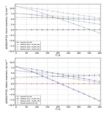
Fig. 8 Variation of the Gibbs energy of the most stable calculated complexes as a function of the temperature computed at the B3LYP-D3(BJ.abc)/ma-def2-TZVP level of theory. The zero of the scale is taken at the most stable insertion structure of each dimer. Solid lines indicate the use of the Rigid Rotor Harmonic Oscillator (RRHO) approximation while dashed lines indicate the use of Grimme's Quasi Rigid Rotor Harmonic Oscillator (QRRHO) approximation.
