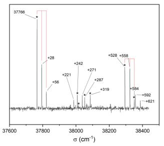
Fig. 3 REMPI  $S_1 \leftarrow S_0$  electronic spectrum of the *cis*-PCD monomer obtained by monitoring its mass at m/z 192 as a function of the laser wavenumber. The 28 cm<sup>-1</sup> progression is materialised by vertical lines. The IR-UV spectra were recorded by setting the probe on the electronic transitions indicated by \*.
