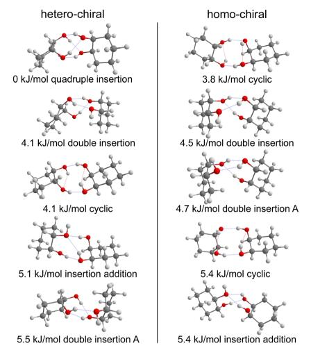
Fig. 13 Five most stable hetero- (left) and homo-chiral (right) dimers of cis-CD, respectively. The zero-point corrected energies at the B3LYP-D3(BJ,abc)/ma-def2-TZVP level are shown. Intermolecular hydrogen bonds are highlighted in blue and intramolecular ones in red.
