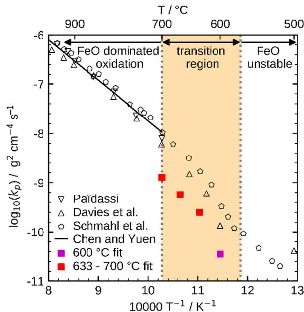
Fig. 10 Comparison of  $K_p$  determined with the present kinetics to reference values from the literature (Païdassi,<sup>21,22</sup> Davies *et al.*,<sup>24</sup> Schmahl *et al.*,<sup>56,61</sup> and Chen and Yuen<sup>13</sup>).
