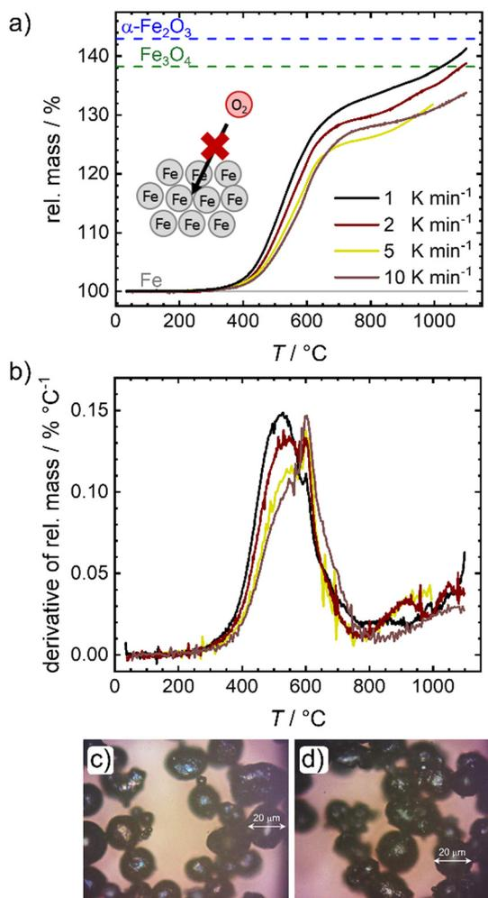
Fig. 2 (a) Temperature programmed oxidation and (b) related derivatives for different heating rates. For reasons of comparison the mass gain assigned to a full oxidation to Fe<sub>3</sub>O<sub>4</sub> and α-Fe<sub>2</sub>O<sub>3</sub> are added. (c) and (d) Photographs of the samples obtained from oxidation under constant heating in a tube oven with 1 K min<sup>-1</sup> up to 300 °C (c) and 600 °C (d).
