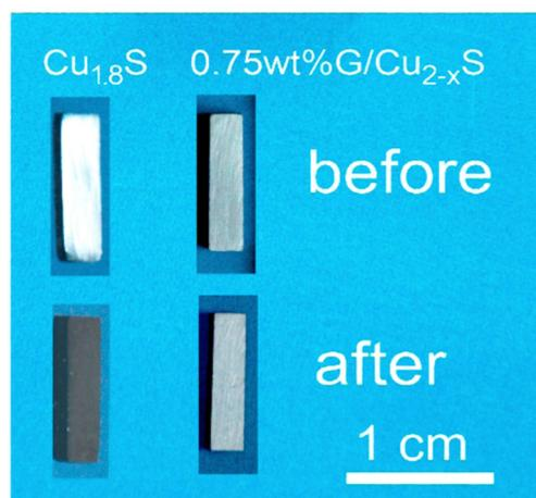
Fig. 6 Photos of the  $\text{Cu}_{18}\text{S}$  before and after high temperature test at 723 K, and 0.75 wt% graphene/ $\text{Cu}_{2-x}\text{S}$  at 873 K, respectively, Reproduced with permission from Ref. 1 Copyright 2018, Elsevier BV.
