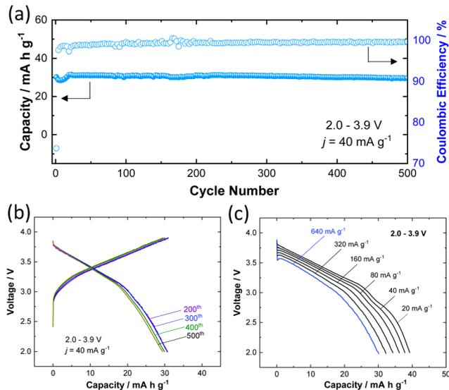
Fig. 4 Electrochemical properties of  $\text{K}_{0.6}\text{Cr}_{0.6}\text{Ti}_{0.4}\text{O}_2$  as a potential positive electrode material for KIBs; (a) cycling stability for 500 cycles in the potential range of 2.0–3.9 V, (b) corresponding charge/discharge curves at the 200th, 300th, 400th, and 500th cycles, and (c) rate capability (active material mass loading:  $2.16 \text{ mg cm}^{-2}$ ).
