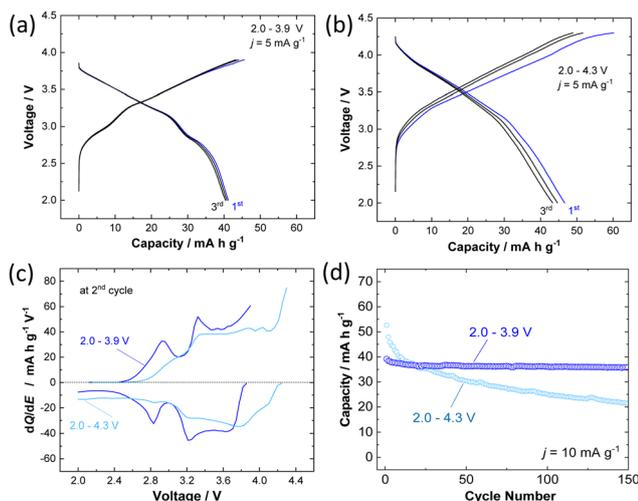
**Fig. 2** Electrochemical properties of  $K_{0.6}Cr_{0.6}Ti_{0.4}O_2$ : (a) the charge/discharge curves of the sample in the potential window range of 2.0–3.9 V at a current rate of  $5 \text{ mA g}^{-1}$ , (b) charge/discharge profiles in the potential window range of 2.0–4.3 V, (c)  $dQ/dE$  plots at the 2nd cycle in the voltage range of 2.0–3.9 V and 2.0–4.3 V, and (d) capacity retention for 150 cycles with two distinct voltage cutoffs at a current rate of  $10 \text{ mA g}^{-1}$ .
