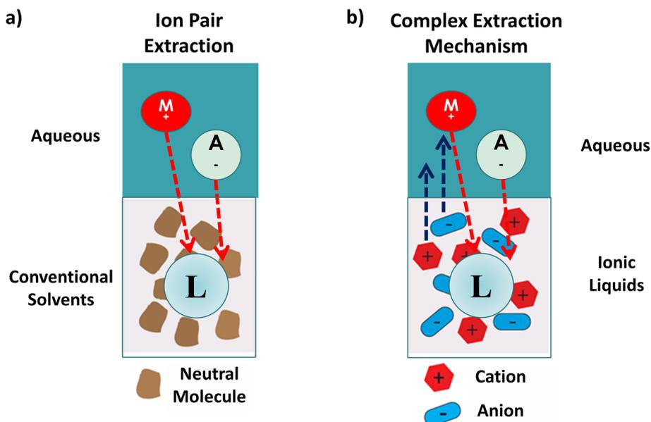
Fig. 1 Liquid-liquid extractions involving (a) conventional organic solvents and (b) ionic liquids.
