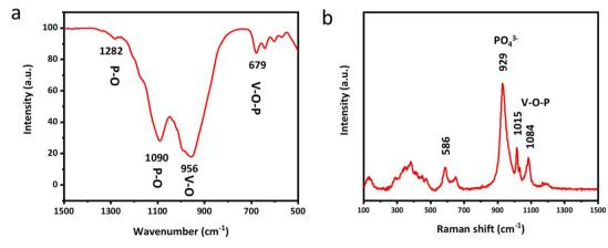
Fig. 2 (a) FTIR spectra and (b) Raman spectra of  $\delta$ -VOPO<sub>4</sub> powder.
