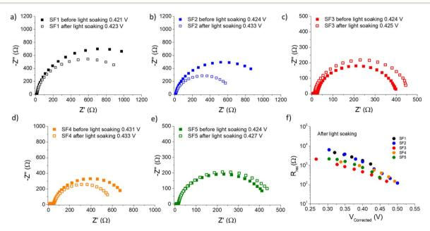
Fig. 5 (a—e) Electrochemical impedance spectroscopy results of SF1-5 dyes solar cells. The Nyquist plots are shown both before and after light soaking. (f) Recombination resistance vs. corrected voltage for SF1-5 dyes under red illumination and after light soaking. Note: the comparison of the recombination resistance vs. corrected voltage for SF1-5 dyes before and after light soaking, can be found in ESI.†
