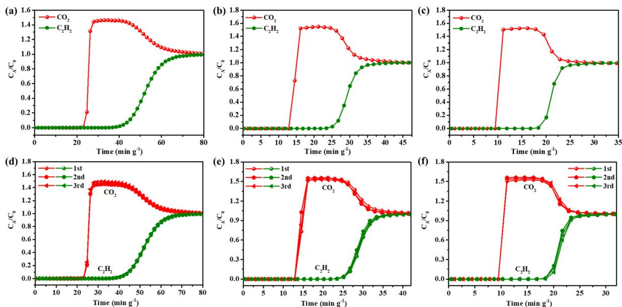
**Fig. 7** Experimental column breakthrough curves for (a)  $C_2H_2/CO_2$  (50/50) mixture under a flow of  $1\text{ mL min}^{-1}$ , (b)  $C_2H_2/CO_2$  (50/50) mixture under a flow of  $2\text{ mL min}^{-1}$  and (c)  $C_2H_2/CO_2$  (50/50) mixture under a flow of  $3\text{ mL min}^{-1}$  in an absorber bed packed with Tb-NTB-1,4-NDC at 298 K and 1.0 bar; (d), (e) and (f) their regenerative tests, respectively.
