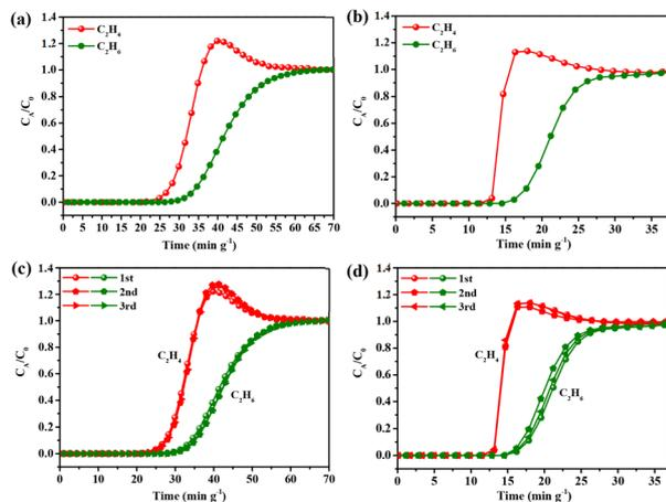
**Fig. 6** Experimental column breakthrough curves for (a)  $C_2H_6/C_2H_4/He$  (25/25/50) mixture under a flow of  $2\text{ mL min}^{-1}$  and (b)  $C_2H_6/C_2H_4/He$  (5/45/50) mixtures under a flow of  $6\text{ mL min}^{-1}$  in an absorber bed packed with Tb-NTB-1,4-NDC at 298 K and 1.0 bar; (c) and (d) their regenerative tests, respectively.
