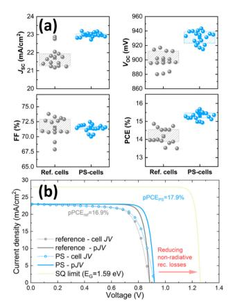
Fig. 4 (a) Short-circuit current density  $(J_{SC})$ , open-circuit voltage  $(V_{OC})$ , fill factor (FF) and power conversion efficiencies of manufactured CPSCs with and without a sacrificial PS laver. (b) JV curves and pseudo-JV curves of the optimum reference and nano-architectured cells, in comparison with the curve at the Shockley-Queisser limit.
