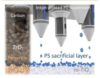
Fig. 1 Conceptual illustration depicting an inkjet-printing process of a sacrificial layer of polystyrene (PS) particles for nano-architectured perovskite solar cells with carbon-based electrodes with a solar cell structure depicted on the left.
