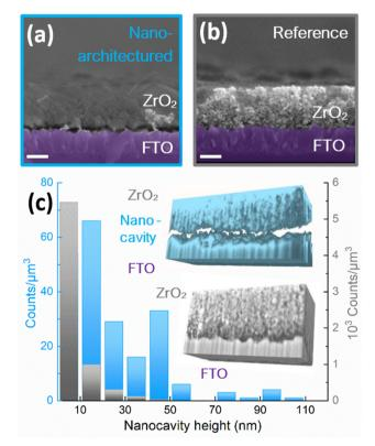
Fig. 2 Cross-sectional scanning electron microscopy (SEM) images of (a) the nano-architectured layer of ZrO<sub>2</sub> and (b) the reference layer of ZrO<sub>2</sub>. Scale bars - 500 nm. (c) Distribution of the cavity height in the nano-architectured (blue) and reference (grey) samples, obtained from 3D-nanotomography using focused ion-beam (FIB) ablation.
