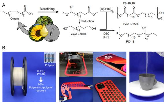
Fig. 12 (A) Biobased materials can be used to make building blocks to make high molecular weight polyethylene-like materials. (B) Polymers can be made into filaments used to 3D print products such as smartphone cases and cups that can hold boiling water while maintaining shape and dimensions. Reproduced in part with permission from ref. 30. Copyright 2021 Nature
