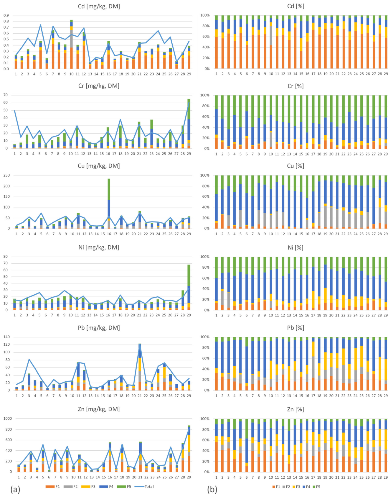
Fig. 4 Fractionation of Cd, Cr, Cu, Ni, Pb, and Zn for all sites (1–29). (a) The graphs to the left are reported as total concentrations ( \text{mg kg}^{-1} , DW), while those (b) to the right report the distribution between fractions (%).
