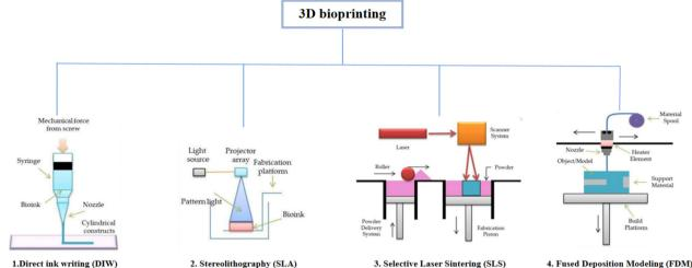
Fig. 3 Classification of 3D printing technology depending on the principle of 3D printing<sup>69</sup> (Copyright © 2021, MDPI).
