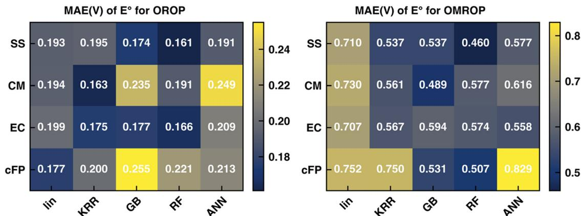
Fig. 2 Test set MAE of the  $\Delta$ -ML corrected redox potential (calculated with PBE0-D3 functional) for (left) OROP and (right) OMROP datasets. The  $\Delta$ -ML models were trained with different combinations of descriptors and ML models.
