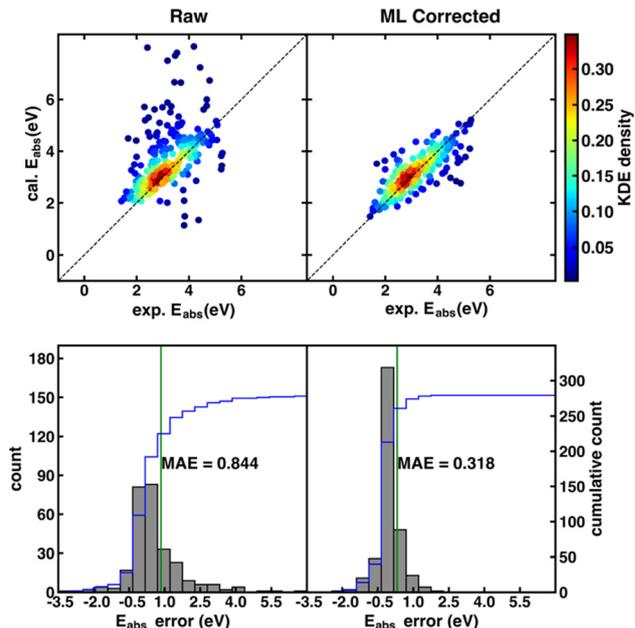
Fig. 3 (top) Parity plots of the PBE0 calculated vs. experimental  $E_{\text{abs}}$ . Top left: Raw data from TD-DFT/TDA calculations. Top right:  $\Delta$ -ML corrected data obtained with the best-performing cFP descriptor combined with the GB model. As indicated by the color bar on the right, data points are colored by kernel density estimation (KDE) density values. (bottom) Histograms of errors of the  $E_{\text{abs}}$  before (bottom left) and after  $\Delta$ -ML correction (bottom right).
