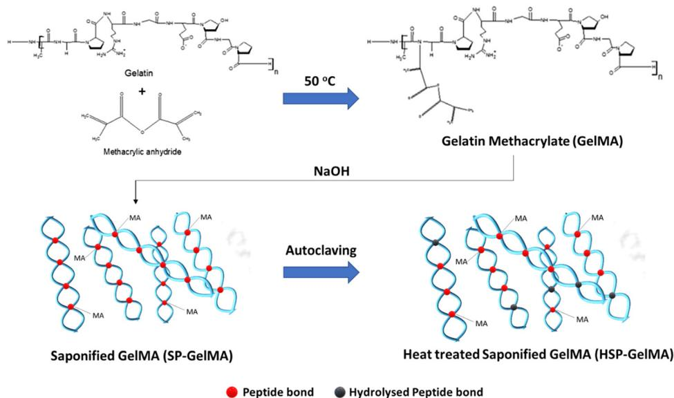
**Fig. 1** Schematic drawing of the two-step modification process for the gelatin methacrylate (GelMA) bio-ink; a saponification process was first performed under highly alkali conditions, followed by the autoclaving process (different numbers of heat treatment cycles) to obtain the heat-saponified GelMA (HSP-GelMA) bio-inks which were illustrated in the macromolecular form.
