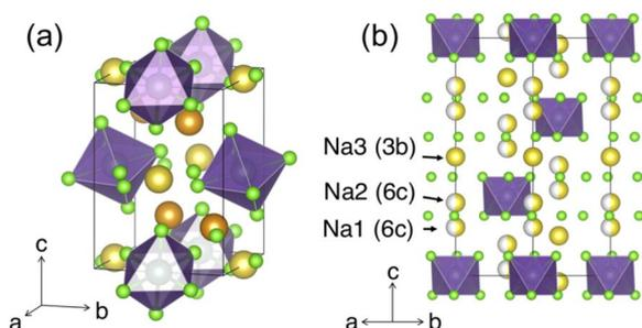
Fig. 4 Polymorphs of the Na<sub>3</sub>YCl<sub>6</sub> composition. Color legend: Y is purple, Cl is light green, while Na atoms in octahedral and prismatic environments are yellow and orange, respectively. (a) The  $P2_1/n$  structure with Na occupying prismatic and octahedral sites. (b) The  $R\bar{3}$  polymorph, as seen down the [110] direction. The three Na sites are depicted with varying degrees of occupancy, as reported by Stenzel and Meyer.<sup>29</sup>
