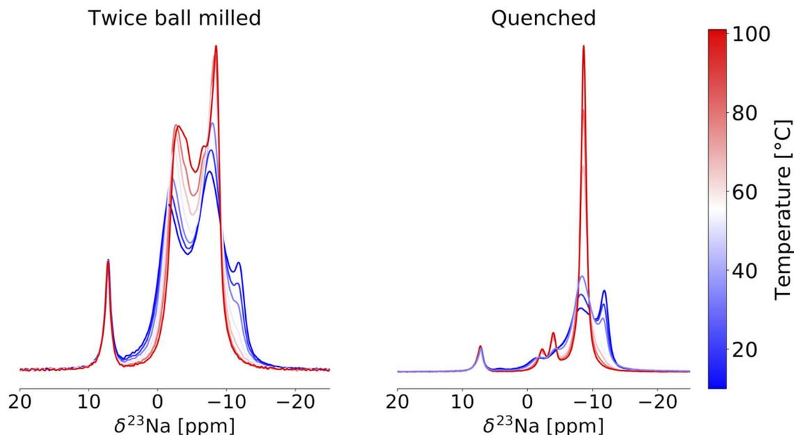
Fig. 9  $^{23}\text{Na}$  variable temperature ss-NMR spectra collected on the twice ball milled (left) and quenched (right)  $\text{Na}_{2.25}\text{Y}_{0.25}\text{Zr}_{0.75}\text{Cl}_6$  samples. Spectra are color-coded using the temperature scale to the right of the plots. The resonance at 7.2 ppm corresponds to NaCl. All spectra were obtained at 18.8 T and at a 10 kHz MAS speed.
