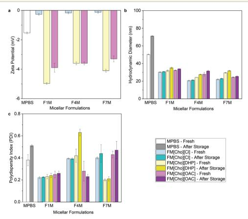
Fig. 3 (a) Zeta-potential values, (b) hydrodynamic diameters, and (c) polydispersity indices of FITC-IgG in micellar-PBS (MPBS) control and select micellar-IL formulations (2 w/w% OBD). Before storage MPBS, FM[Cho][Cl], FM[Cho][DHP], and FM[Cho][OAC] are represented by white, faint blue, faint yellow and magenta, respectively, and after storage by grey, cyan, dark yellow, and purple, respectively. For all micellar-IL formulations see Tables S1 and S3.†
