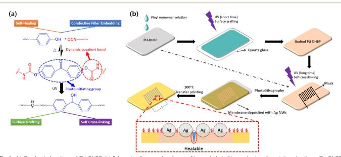
Fig. 1 (a) Quadruple functions of PU-DHBP. (b) Schematic diagram of surface grafting and photolithography-transfer printing circuits on PU-DHBP. Based on dynamic phenol-carbamate bonds and benzophenone units, PU-DHBP can realize various functions such as self-healing, repeated processing, surface grafting, self-crosslinking, embedding conductive fillers, etc
