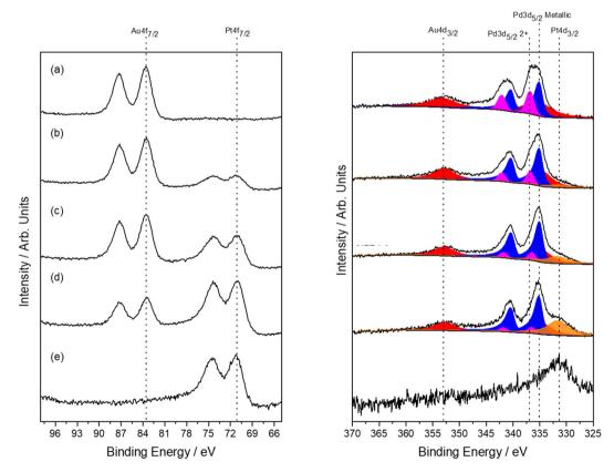
Fig. 6 XPS Au(4f)/Pt(4f) and Pd(3d)/Au(4d) spectra for as-prepared 0.66%AuPdPt/TS-1 catalysts, prepared by sol-immobilisation (PVA: metal = 1.2). (a) 0.33%Au-0.33%Pd/TS-1, (b) 0.275%Au-0.275%Pd-0.11%Pt/TS-1, (c) 0.22%Au-0.22%Pd-0.22%Pt/TS-1 (d) 0.11%Au-0.11%Pd-0.44%Pt/TS-1 and (e) 0.66%Pt/TS-1. Note: all catalysts were exposed to an oxidative heat treatment prior to use (static air, 400 °C, 3 h).
