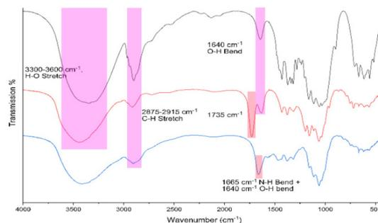
Fig. 1 FTIR spectrum of pristine cellulose nanocrystals derived from cotton by sulfuric acid hydrolysis (black), chlorinated CNCs from  $\text{SOCl}_2$  in DMF (red) and TAEA-modified cellulose (blue).
