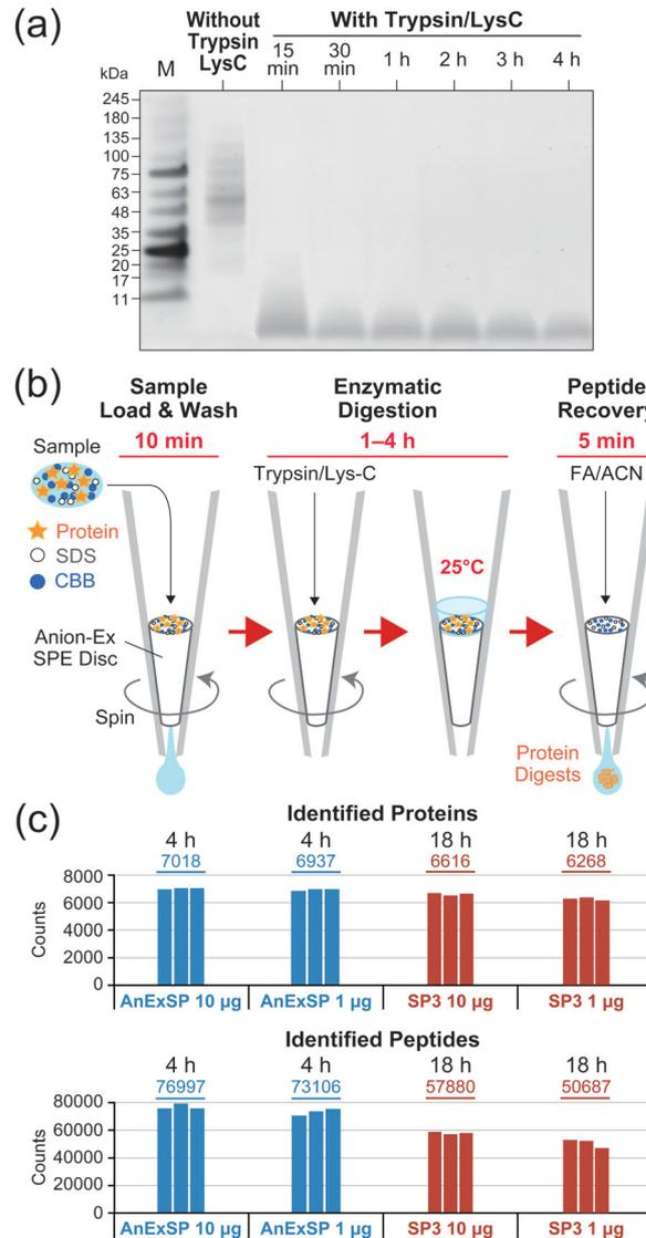
**Fig. 1** Sample pretreatment for bottom-up MS using AnExSP. (a) SDS-PAGE of digested HCPE recovered from AX SPE discs. After digestion of HCPE with Trypsin/Lys-C, digestion products recovered from AX SPE discs with 10% SDS were separated by SDS-PAGE and visualized with CBB. The substrate enzyme ratio was set to 20:1. M: molecular weight marker. (b) Schematic workflow of AnExSP. FA: formic acid. ACN: acetonitrile (c) DIA analysis of digestion products.
