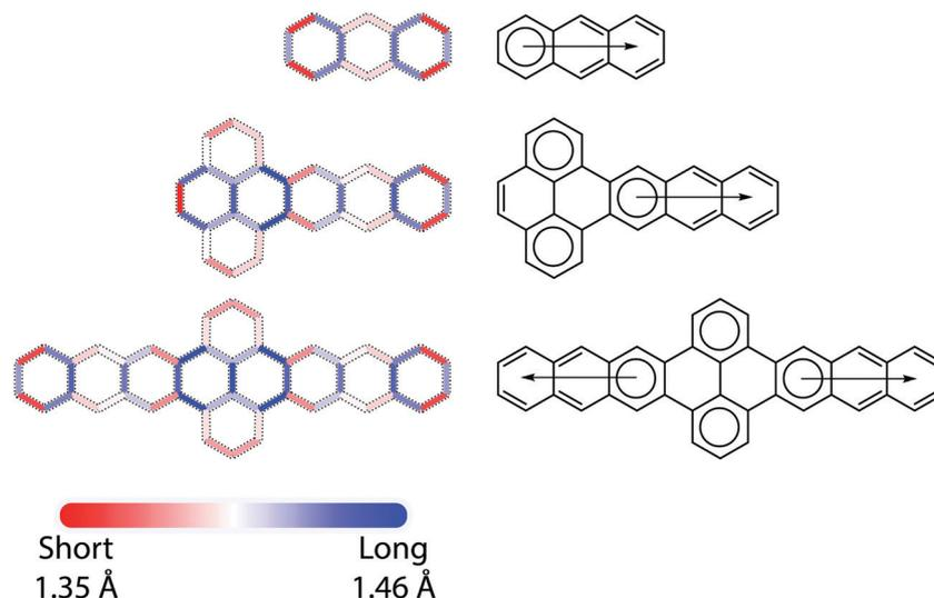
Fig. 2 (Left) Bond length alternation (BLA) patterns of, from top to bottom, anthracene, P-A3, A3-P-A3 as determined at the LC- $\omega$ HPBE/Def2TZVP level of theory. Only the C-C bonds in the molecular backbones are shown. (Right) Corresponding Clar formulae of these molecules.
