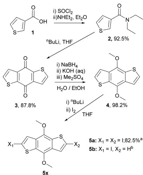
**Scheme 1** The synthetic route and yields to common benzodithiophene intermediates **5a** and **5b**. <sup>a</sup>Yield for reaction on 1 g scale, <sup>b</sup>Isolated as a side product from the reaction on 100 g scale.
