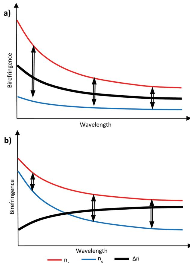
Fig. 2 Graphical representation of (a)  $n_o$  is smaller and less wavelength dependant giving positive dispersion and (b) when  $n_o$  is larger and more wavelength dependant giving negative dispersion.
