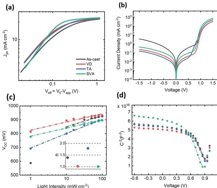
Fig. 4 (a) Photocurrent density ( $J_{PH}$ ) as a function of effective voltage ( $V_{eff} = V_0 - V_{app}$ ). (b) Dark  $J$ - $V$  curves. (c) Open-circuit voltage as a function of light intensity; the inset shows the diode ideality factor ( $n$ ). (d) Capacitance as a function of applied voltage.
