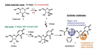
Scheme 1 Synthetic approaches to uprifosbuvir 1 with the two main challenges highlighted. (a)  $Me_2NH$ , AcOH, EtOH/MeOH, 80 °C, 1.5 h; (b)  $Ca(OH)_2$ , water, 70 °C, 24 h, 19% over 2 steps.<sup>9</sup>
