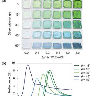
**Fig. 5** (a) Photographs at different viewing angles of films prepared from aqueous dispersions of Wp2 with various amounts of Bp1-h. (b) Absolute specular reflectance UV-vis spectra of a cast film containing Wp2 and 5 wt% of Bp1-h. Both the incident angle and the detection angle were set to the specified angles (f).
