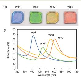
Fig. 6 (a) Photographs of colloidal crystal films of Wp1 (212 nm), Wp2 (240 nm), Wp3 (261 nm), and Wp4 (270 nm) with 1 wt% of Bp1-h. (b) Diffuse reflectance UV-vis spectra of films containing each type of colloidal silica nanoparticle and 1 wt% Bp1-h.
