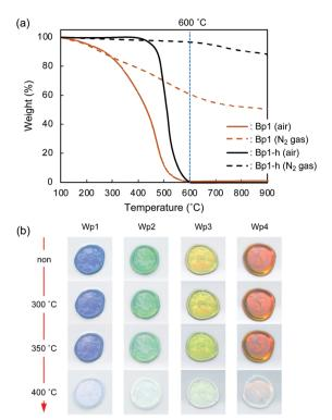
(a) TGA measurements of  $\pi$ -conjugated polymer nanoparticles (Bp1) and black carbon nanoparticles (Bp1-h) under air and N2 gas atmospheres. Heating rate: 10 °C min<sup>-1</sup>. Gas flow rate: 200 mL min<sup>-1</sup>. (b) Thermal stability of structural colours from the silica nanoparticle (Wp1 to Wp4)-based colloidal crystals doped with 1 wt% Bp1-h.
