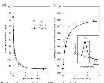
Fig. 4 (a) Baseline reflectance (680 nm, a) and (b) the relative peak intensity at  $\lambda_{\rm max}$  (b/c) after doping black carbon nanoparticles at different concentrations.
