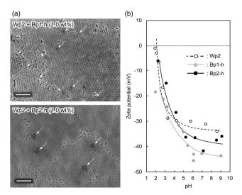
Fig. 3 (a) FE-SEM images of the colloidal crystal of silica nanoparticles (Wp2) with 1 wt% black carbon nanoparticles (Bp1-h and Bp2-h). Scale bars: 2 µm. (b) Zeta potentials of the aqueous dispersions of Wp1, Bp1-h, and Bp2-h in a wide pH range
