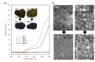
Fig. 1 (a) Diffuse reflectance UV-vis spectra and (b) FE-SEM images of  $\pi\text{-conjugated}$  polymer nanoparticles before (Bp1 and Bp2) and after (Bp1-h and Bp2-h) heat treatment. The insets in (a) are the photographs of the particles. Heat treatment was carried out at 600  $^{\circ}\text{C}$  under N $_2$  gas for 2 h. Scale bars in (b): 2  $\mu\text{m}$ .
