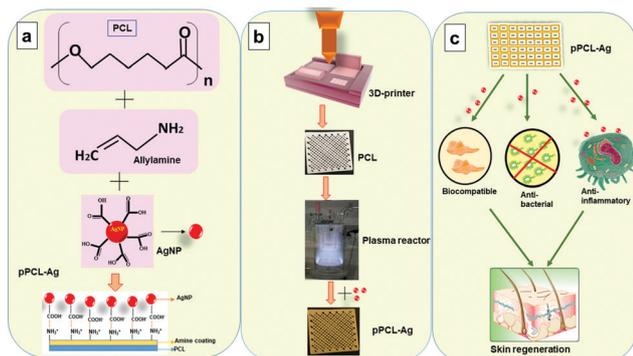
Fig. 1 Schematic representation of (a) the components involved in the fabrication of plasma polymer-modified PCL scaffolds containing AgNPs (pPCL-Ag) and their chemistry of immobilisation; and processes involved; and (c) targeted outcomes.
