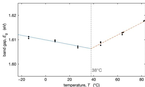
Fig. 5 Band gap (eV) (black dots) for perovskite composition  $\text{Cs}_{0.17}\text{FA}_{0.83}\text{Pb}(\text{Br}_{0.17}\text{I}_{0.83})_3$  as a function of temperature (°C), calculated from up and downward cycles of EQE, with a linear fit before discontinuity (blue dashed line) and after slope discontinuity (red dotted line). The grey dashed line shows the intersection of the two fit slopes.
