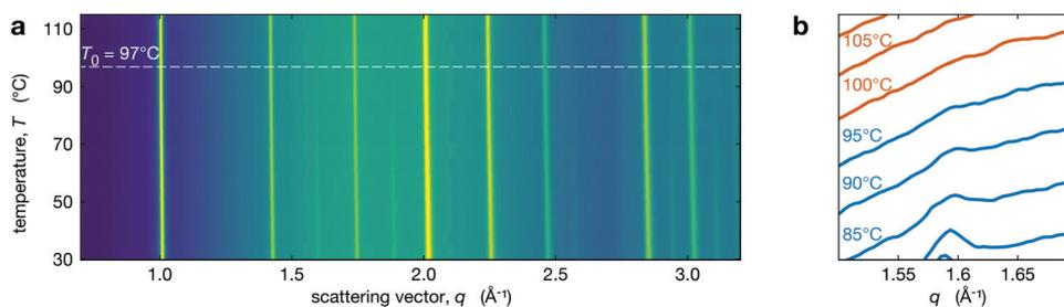
**Fig. 2** (a) Temperature XRD map for  $\text{Cs}_{0.4}\text{FA}_{0.6}\text{Pb}(\text{Br}_{0.17}\text{I}_{0.83})_3$  with the extracted  $T_0$  (temperature where film is purely cubic) indicated by a dashed line. (b) Evolution of the integrated intensity of the  $t(210)$  superlattice peak. Temperature is increasing moving up in the vertical direction. The y-axis is linear and represents the intensity counts in arbitrary units.
