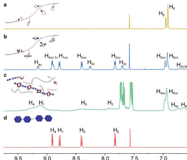
Fig. 2 Partial <sup>1</sup>H NMR (400 MHz, CD<sub>3</sub>CN:CDCl<sub>3</sub> = 3:1 v/v, 298 K) of (a) CP-1, (b) CP-2, (c) CSP-2 and (d) the bis(pyridinium) ligand. Letters "c" and "uc" denote complexed and uncomplexed species, respectively.
