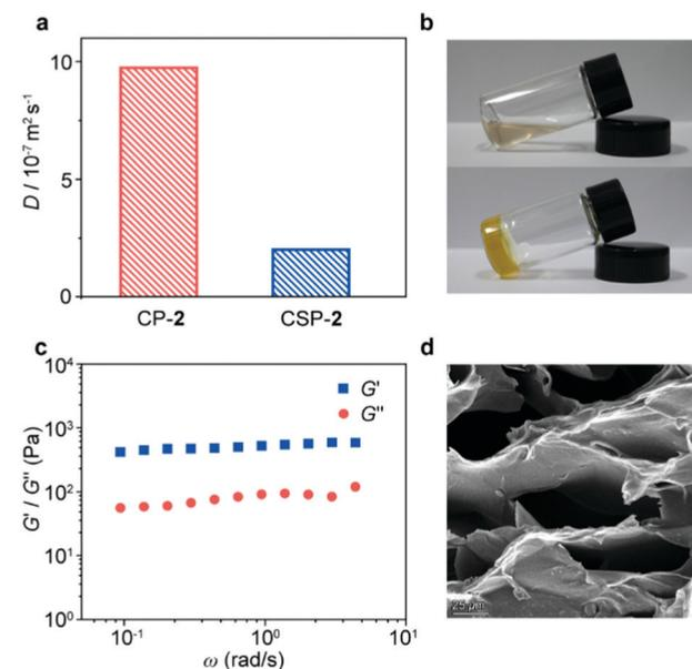
Fig. 3 (a) Diffusion coefficient  $D$  (500 MHz, CD<sub>3</sub>CN/CDCl<sub>3</sub> = 3:1 v/v, 298 K) of CP-2 and CSP-2. (b) Images of CP-2 solution (above) and CSP-2 gel (below). Solvent: CH<sub>3</sub>CN:CHCl<sub>3</sub> = 3:1 v/v, 2.0 mL. (c) Storage modulus  $G'$  and loss modulus  $G''$  versus frequency  $\omega$  for the CSP-2 gel. (d) The SEM image of the freeze-dried CSP-2.
