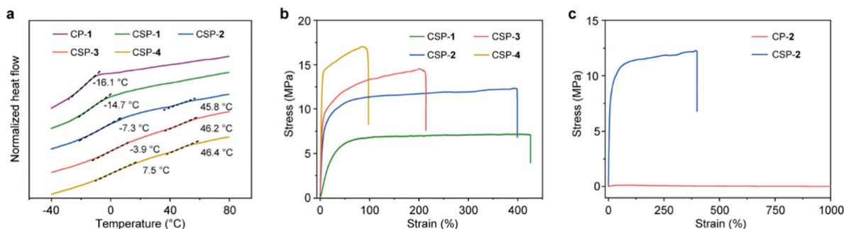
Fig. 4 (a) DSC curves of CP-1 and CSPs-1–4 recorded by heating scan from -40 to 80 °C with a heating rate of 20 °C min<sup>-1</sup>. (b) Tensile stress–strain curves of CSPs-1–4 in the bulk. Deformation rate: 20 mm min<sup>-1</sup>. (c) Tensile stress–strain curves of CP-2 and CSP-2 samples in the bulk. Deformation rate: 20 mm min<sup>-1</sup>.
