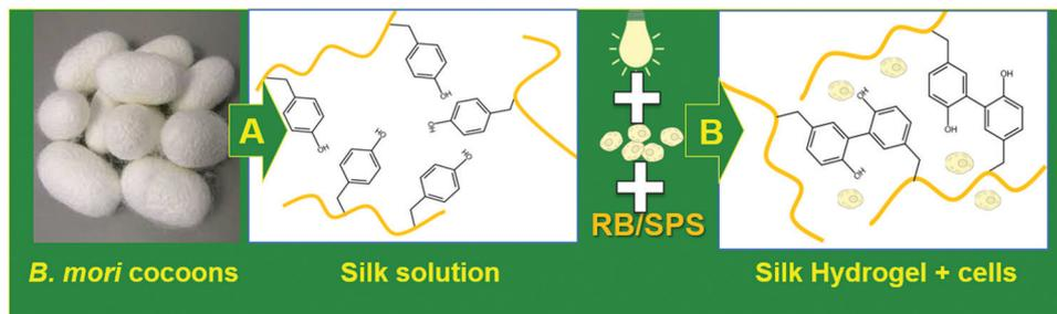
**Fig. 1** Schematic of the fabrication of cell-laden silk fibroin hydrogels (A). In a first step (A), silk fibroin aqueous solutions extracted from cocoons are mixed with cells, followed by riboflavin (RB) and sodium persulfate (SPS). Exposure to visible light promote hydrogel formation through di-tyrosine crosslinks (B).
