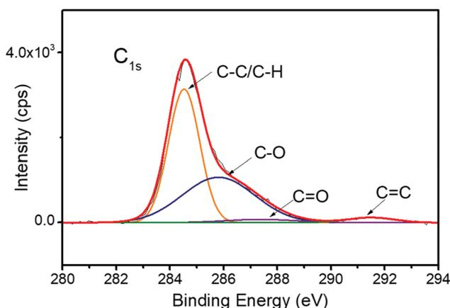
Fig. 4 XPS spectrum of P(VGal<sub>10%</sub>-co-St<sub>90%</sub>) remained on fractured surface after adhesion tests.
