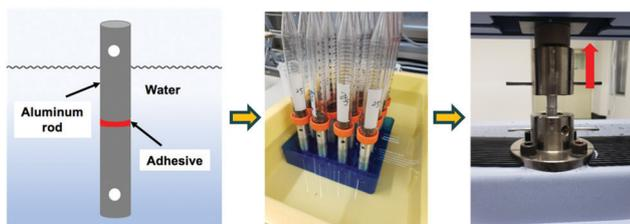
**Scheme 2** Experimental process for measuring underwater adhesion strength. The polymer solution was applied underwater and cured for a certain period. The samples were taken out from water and tested immediately.
