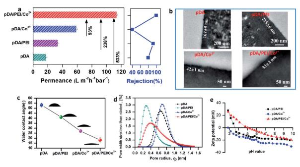
Fig. 2 (a) Permeance and (BTB) rejection results; (b) TEM images; (c) water contact angles (WCAs); (d) the pore size distribution; (e) zeta potentials of the binary (pDA/PEI and pDA/Co $^{2+}$ ) and ternary (pDA/PEI/Co $^{2+}$ ) coated membranes.
