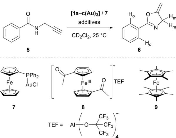
Scheme 2 Gold(I)-catalysed ring-closing isomerisation of *N*-(2-propyn-1-yl)benzamide **5** to oxazoline **6** (top, labelled protons used for following the reaction), including alternative mononuclear (pre-) catalyst **7**, oxidant **8**, and reductant **9**.
