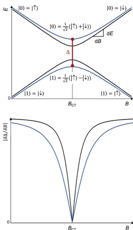
Fig. 1 (Up) Anticrossings between pairs of states with equal Zeeman slopes  $dE/dB$  but either large (blue) or a small (black) tunneling splitting  $\Delta_{CT}$ . (Down) Sensitivity to the magnetic field  $|\partial\Delta/\partial B|$ , near the anticrossings: in the black curve the protection is lost quickly whereas a larger  $\Delta_{CT}$  means a relatively wide window of protection for the blue curve.
