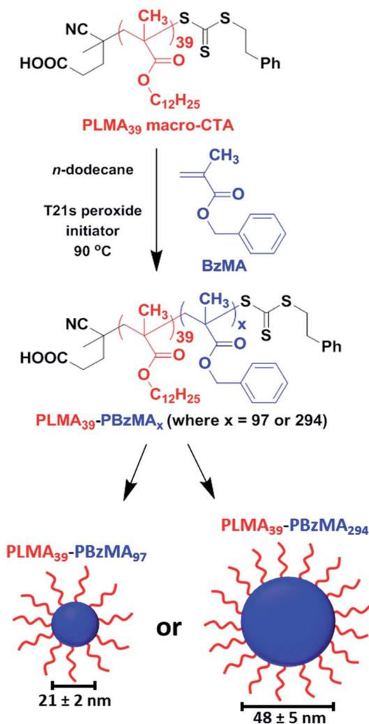
**Scheme 1** A PLMA<sub>39</sub> precursor block is chain-extended with BzMA monomer in *n*-dodecane via RAFT-mediated PISA to form sterically-stabilized spherical nanoparticles. SAXS analysis (see Fig. S3, Tables S2 and S3 in the ESI†) indicated that final PBzMA DPs of 97 and 294 produced mean core diameters of 21 ± 2 nm and 48 ± 5 nm, respectively.
