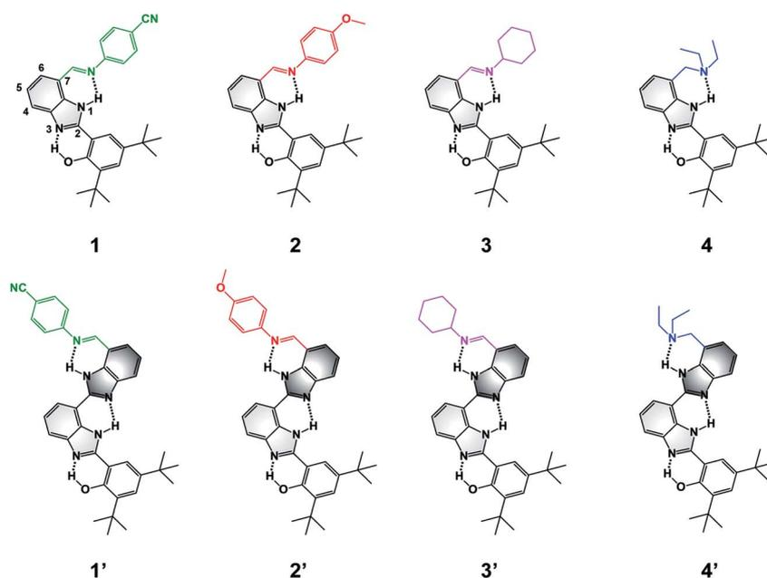
Fig. 1 Molecular structures of BIP (**1–4**) and BI<sub>2</sub>P (**1'–4'**) constructs bearing different terminal proton-accepting groups (color-coded as in Fig. 4–6). The numbering system is shown in **1**, and the incorporation of a second benzimidazole to form dibenzimidazole based bridges between the phenol moiety and the terminal proton-accepting group are shown in dark grey in **1'–4'**.
