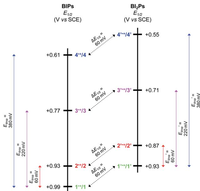
Fig. 5 Diagram showing the experimentally determined  $E_{1/2}$  for BIP derivatives (1–4) and BI<sub>2</sub>P analogs (1'–4'). The colored arrows show that the drop in  $E_{1/2}$  ( $E_{\text{drop}}$ ) for the different TPAs is the same in both series. The dashed black arrows indicate the decrease in  $E_{1/2}$  ( $\Delta E_{1/2}$ ) due to the addition of one benzimidazole unit, which is 60 mV regardless of the TPA.
