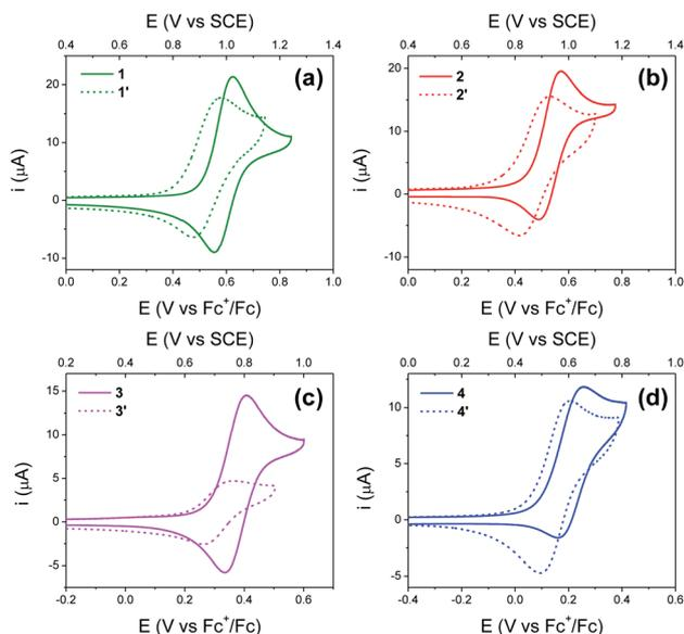
Fig. 4 (a–d) Cyclic voltammograms of Bl<sub>2</sub>P<sub>s</sub> 1'–4' (dashed lines). The cyclic voltammograms of analogous BIPs 1–4 (solid lines) are included for comparison. Concentration: 1 mM of the indicated compound, 0.5 M TBAPF<sub>6</sub> supporting electrolyte in dry acetonitrile. WE: glassy carbon. Pseudo RE: Ag wire (ferrocene as internal reference). CE: Pt wire. Scan rate, 100 mV s<sup>-1</sup>. Compound 3' has low solubility in acetonitrile.
