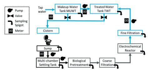
Fig. 1 Flow diagram of the CLASS.
