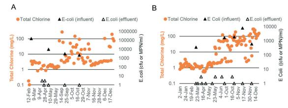
Fig. 6 *E. coli* levels in the blackwater and treated water *versus* total chlorine at sites A and B indicated disinfection. Bacterial counts in the treated water were measured by plate counting (1 CFU per ml resolution) and MPN methods (3 MPN per ml resolution).
