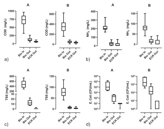
Fig. 4 Water quality parameters [a) COD, b) NH<sub>3</sub>, c) TSS, and d) E. Coli] before biological pretreatment (Bio In), after biological pretreatment (Bio Out), and after electrochemical disinfection (ECR out); lines in the boxes represent medians, the boxes are the 25th and 75th percentiles, and the error bars are the minimum and maximum values. For the numerical values and sample sizes (n), see Table S5.†
