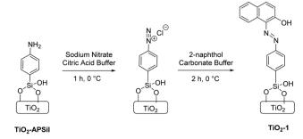
Scheme 2 Diazo coupling reactions to form TiO2-1 including diazotization in the first step and 2-naphthol coupling in the second step.
